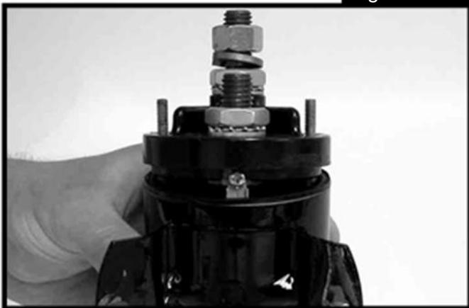
the link spool in the switch plunger and torque to 54-66 lbf-in. Grip the plunger either in soft jaws in a vise or using a pipe wrench and a strip of emery cloth to grip the plunger. Ensure that no nicks or burrs are raised during this operation. Figure 28
