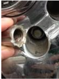
Gambar Baut Roda pecah
