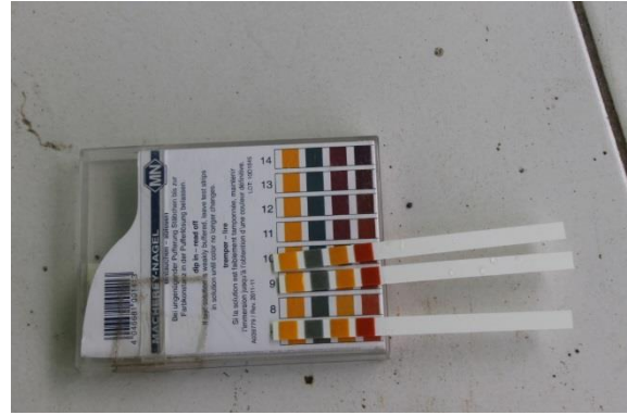
pH measurement in each observation pond
